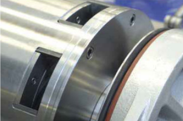
Figure 3. Solids discharge, free from blocking
